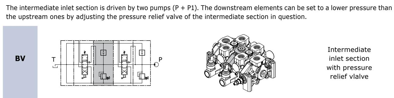
The intermediate inlet section and the elements are driven by a single pump ( $P$ ). The downstream elements can be set to a lower pressure than the upstream ones by adjusting the pressure relief valve of the intermediate section in question.
