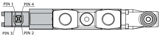
**CONTROL in A e B** = connect PIN 1 - 4 and 2 - 3 - 4
